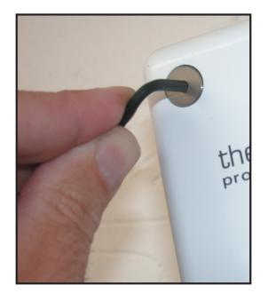
Screw the head screws down with the 3mm allen key provided
